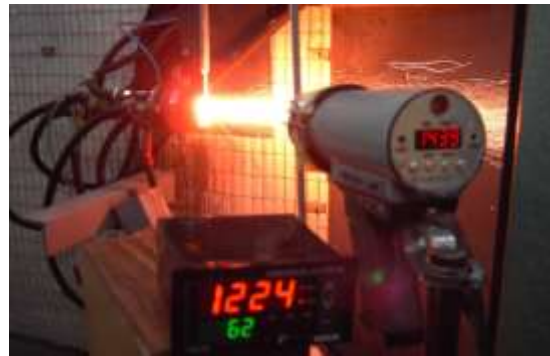
Figure 3: Plasma jet (on the left, without the supply of WCS; on right, with the feed of WCS.)
